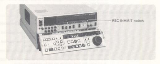
Set the REC INHIBIT switch on the sub control panel to OFF to enable recording. Or, check that recording is not inhibited on the inserted cassette.
